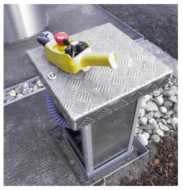
Retractable control column with control bulb
